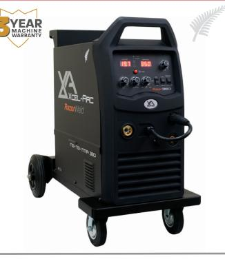
**Technical Data** Power Supply 415V 3-Phase +/- 15% Rated Input Power MIG 13.9 kVA Rated Input Power MMA 15.0 kVA I ieff as per AS/NZ60974-1 13.2 Amps I Max 20.9 Amps Output Current Range MIG 50A/16.5V - 350A/31.5V TIG 20A/10.8V - 350A/24.0V 20A/20.8V - 350A/34.0V MMA Duty Cycle @ 40°C as per AS/NZ60974-1 40% @ 350 Amps MIG 40% @ 350 Amps TIG 40% @ 350 Amps MMA 70% @ 350 Amps MIG Duty Cycle @ 25°C (approximate)
